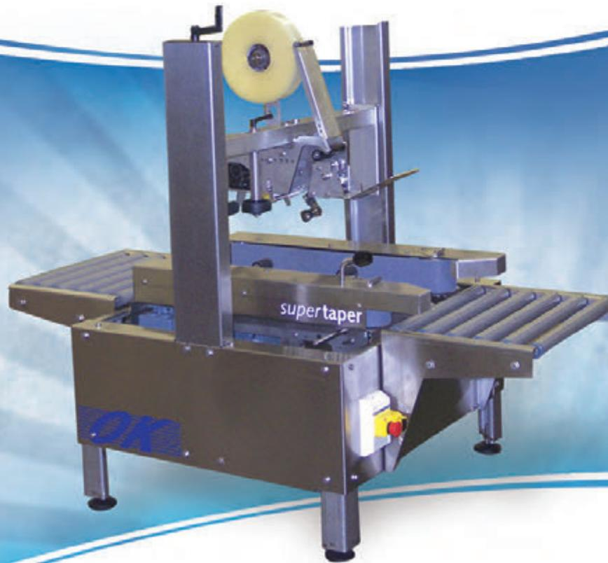
The Supertaper ST1M seals cases on the top and bottom with tape. Features include: stainless steel exterior finish, high-quality taping heads with open tape feed path, heavy duty side belts with 1/4 hp motors and quick and easy size change.
