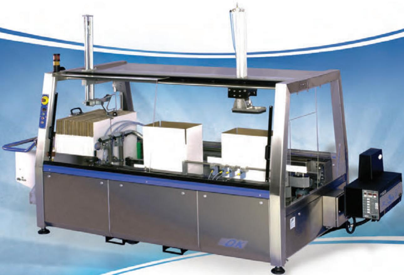
The Superformer SF1-HM erects corrugated cases and closes the bottom flaps with hot-melt glue. Unique features of the machine include stainless steel exterior finish, automatic case squaring system, easy size change, case monitoring, and display with fault finding indications.
