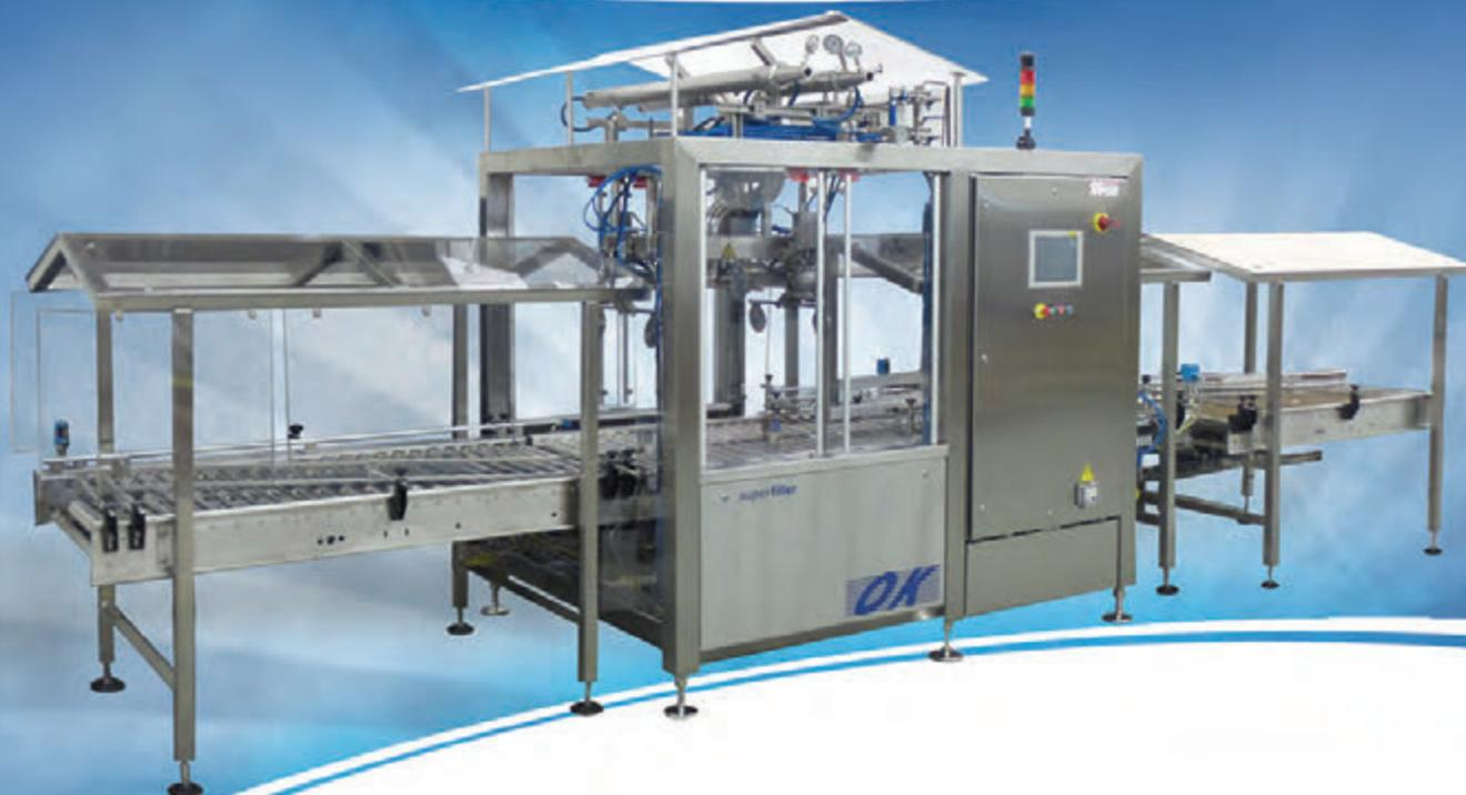
The Superfiller SR4 is a four head Bulk Weighfiller designed for semi-liquid oils and fats, such as shortening and margarine. Also available in a single head model, the Superfiller SR1L and a two head model, the Superfiller SR2.
